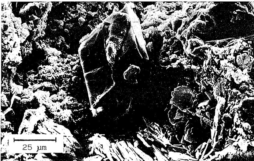
Figure 2.- SEM micrograph of the Bicorp tuff (BIC-5). Sanidine crystal in a fine grained matrix of sanidine and zeolite.
